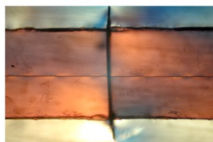
Carbon fiber and phenolic matrix cracks inside epoxy matrix
